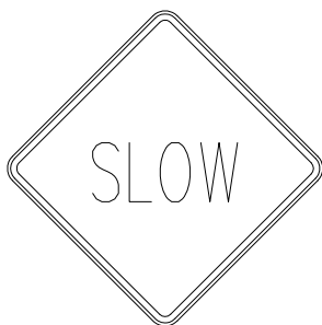
T-2 300mm x 300mm B/Y - HI SIGN GRADE ALUMINIUM - 2mm/.081 9.5mm HOLES. CENTERED, CROPPED CORNERS
