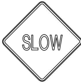
T-2 300mm x 300mm B/Y - DIAMOND GRADE REFLECTIVE SHEET ALUMINIUM - 2mm/.081 9.5mm HOLES. CENTERED, CROPPED CORNERS
