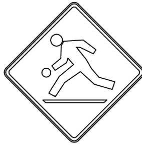
T-14 450mm x 450mm B/Y DIAMOND GRADE REFLECTIVE SHEET. ALUMINUM - 200/0.081 Ø 9.5 ON CENTRE, LARGE CROP.
