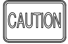
T-16 450mm x 350mm B/Y DIAMOND GRADE REFLECTIVE SHEET. ALUMINIUM - 200/0.081 Ø 9.5 ON CENTRE, LARGE CROP.
