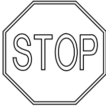
T-1 300mm x 300mm W/R - DIAMOND GRADE REFLECTIVE SHEET ALUMINIUM - 2mm/.081 9.5mm HOLES. LARGE CROPPED CORNERS
