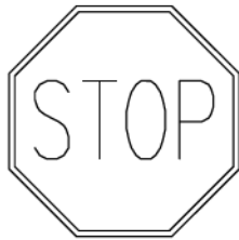
T-1 300mm x 300mm W/R - HI SIGN GRADE ALUMINIUM - 2mm/.081 9.5mm HOLES. LARGE CROPPED CORNERS
