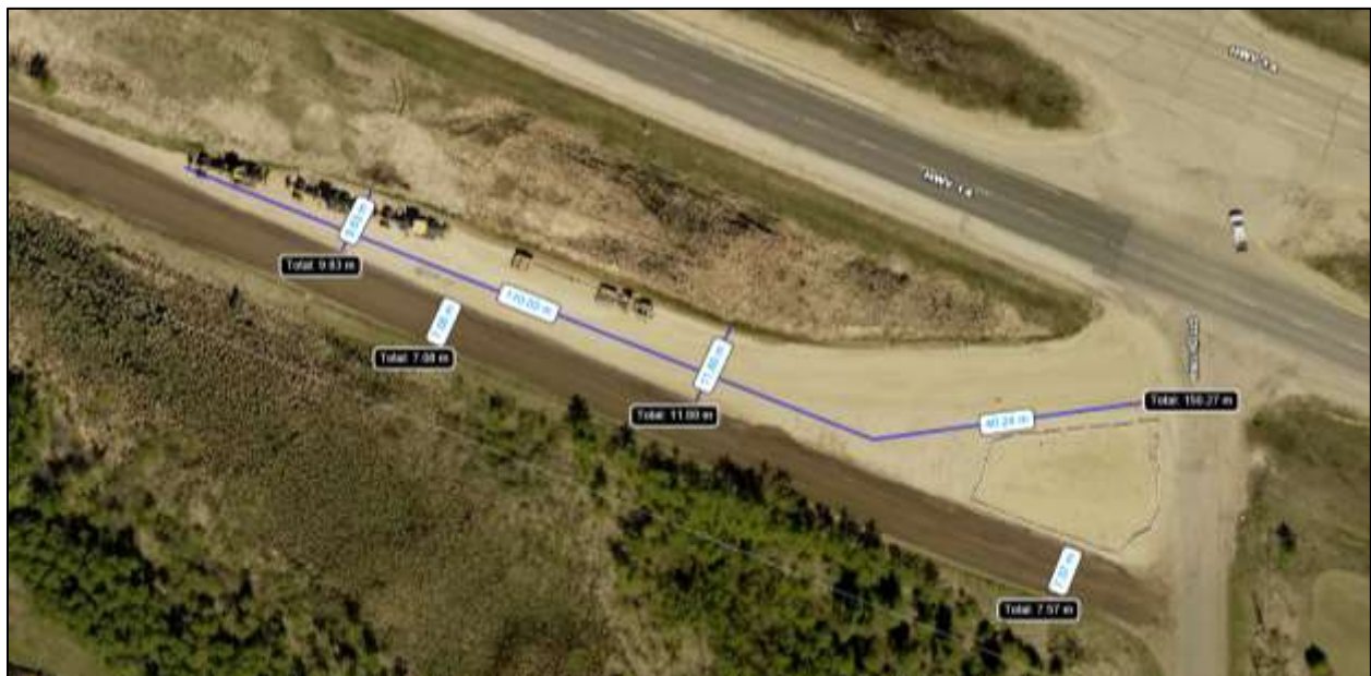
OSOW Staging Area on Highway 14 service road west of Range Road 225 (circa 2017) clearly distinguished between a freshly dust-suppressed 7.0 to 7.5 metre wide service road and an untreated gravel staging area.
