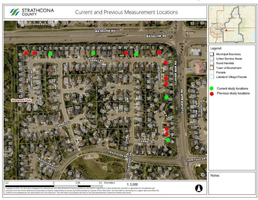
Administration selected five previously unmeasured properties; three along Baseline Road and two along Clover Bar Road, to conduct 24hour noise measurements
